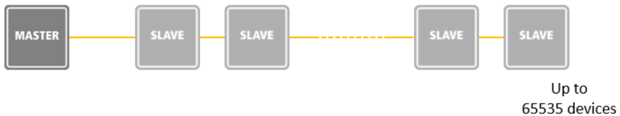
Figure 1: number of slaves on an EtherCAT network
