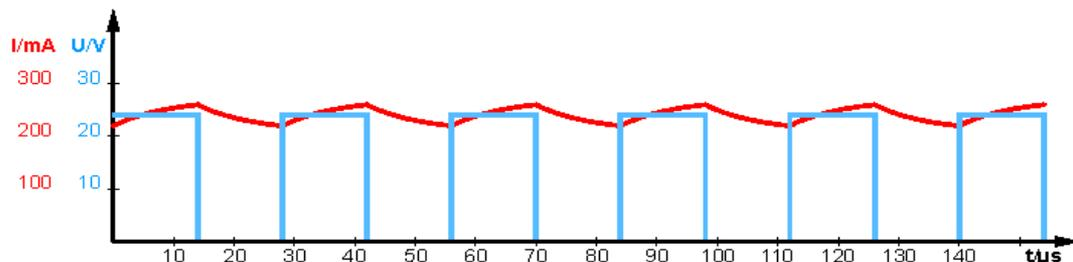
Fig. 1: Operation at load with adequate inductance
