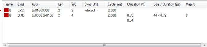
(Example: in case of wrong Working Counter for the LRD datagram, all Slaves Add (Internal Use) ressed by this datagram will set WcState = 1. Reading the State variable of these slaves the master application can investigate which slave is responsible for the error).
