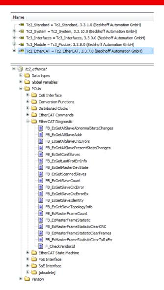
The **TcEtherCAT.lib** library (available free-of-charge with both the default installation of TC2 and TC3) provides function-blocks which enable to acyclically diagnose the EtherCAT network
