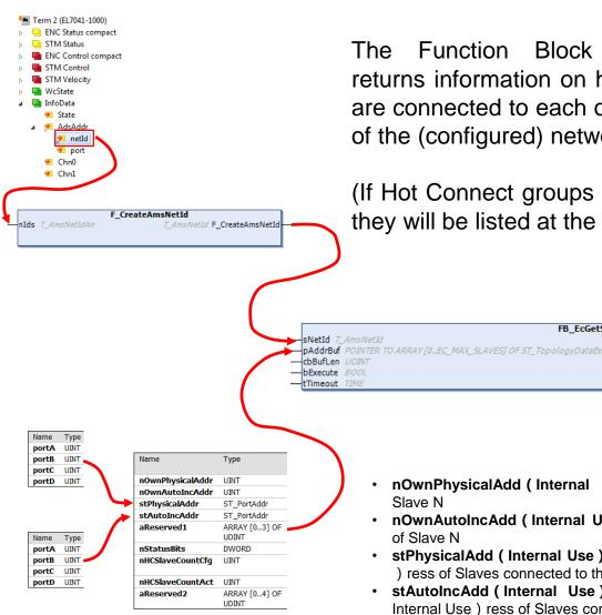
The Function Block **FB\_EcGetSlaveTopologyInfo** returns information on how the ports of different slaves are connected to each other, and therefore the structure of the (configured) network topology.
