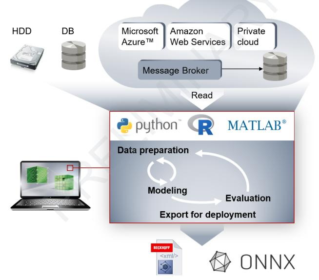
The model learned now has to be exported out of the selected ML Framework and used in the ML Runtime within the TwinCAT Runtime. For this, Beckhoff supports the standardized Open Neural Network Exchange format (<u>ONNX</u>) on the one hand and two of its own proprietary formats on the other. The proprietary formats are firstly a readable XML format and secondly, for the delivery, a binary data format (BML). Read more about the formats here: <u>Supported file formats</u> [▶ <u>26</u>].
