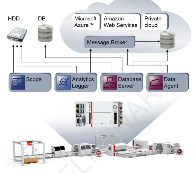
In the engineering phase, the <u>TC3 Scope</u> with its <u>storage function</u> as binary file, CSV, TDMS and other formats is a simple and flexible tool for collecting and storing data. The tool can be used intuitively and quickly via the user interface of the Scope View. The Scope Server can also be controlled directly from the PLC via the PLC function block FB\_ScopeServerControl (Tc2\_Utilities library) and thus used precisely in terms of time as well as reproducibly.
