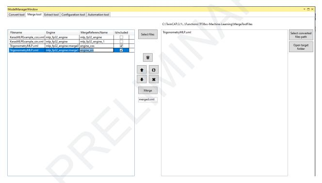
The name of the merged ML description file can be entered in the textbox in the central section. The file is generated with **Merge** and saved in the file path *<TwinCATPath>\Functions\TF38xx-Machine-Learning \MergeToolFiles*. The path can be changed with **Select target path**.
