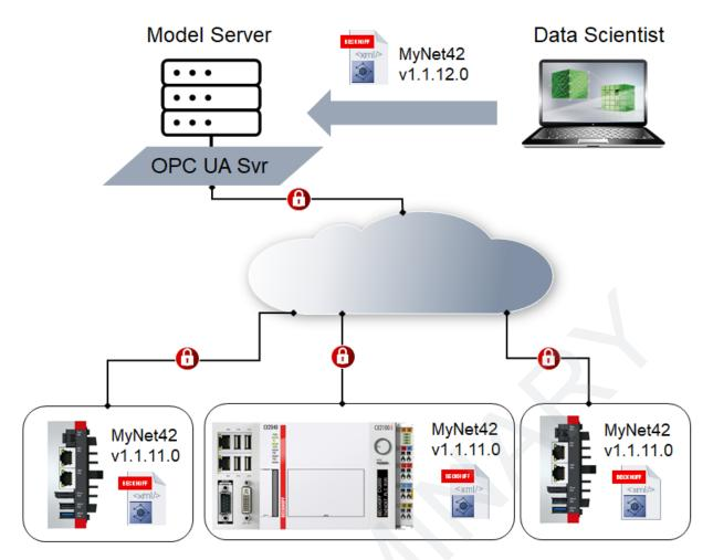
In this case the OPC UA server is implemented on the Model Server side. Appropriate software products for this are available on the market. The OPC UA client can be implemented on the device side and, as in the HTTPS scenario, send requests to the server.
