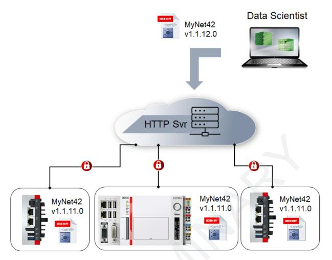
An important difference between this and the MQTT scenario is that a "push" to devices cannot be executed directly starting from the model server unless an incoming HTTPS port is opened. In order to get around this, a device can, for example, request updates cyclically. As with MQTT a payload is not defined, therefore both status information and the model file itself can be transmitted by HTTPS.
