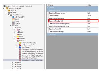
> Define the limit for the mover detection current
