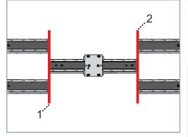
With movable track sections, a double-sided air gap 1 and 2 is required between moving and stationary track sections. The nominal air gap is 1.0 mm and must not exceed 3.0 mm.
