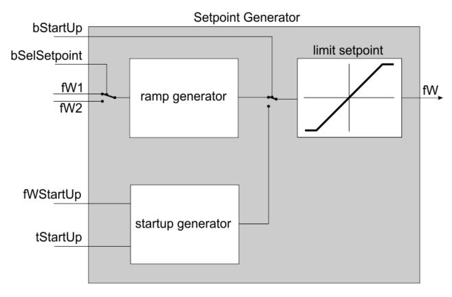
In order to permit "heater baking", a soft start can be parameterized. In this case, the temperature is first ramped up from ambient to a low setpoint (fWStartUp). This temperature is then maintained for a period of time (tStartUp), and only after that has elapsed does the ramp up to the actual setpoint begin.
