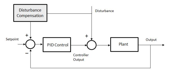
The disturbance compensation is a lead/lag compensator. A lead/lag compensator is a versatile component that can be used to set up I, D, PI, PD, and PID compensations provided the gain and time constants are carefully selected. With the help of the compensator, permanent deviations and peaks can be reduced and the dynamic behavior in case of interference can be improved. Here you can find further information about the lead/lag compensator.
