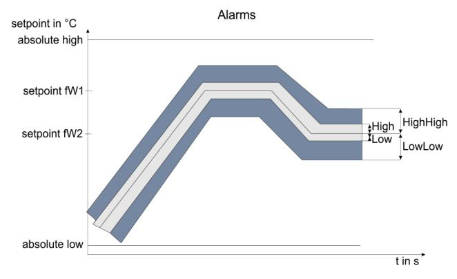
The following alarm conditions are continuously monitored by the temperature controller:
